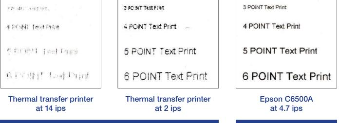
Printed on matte thermal transfer media at best settings using wax ribbon
