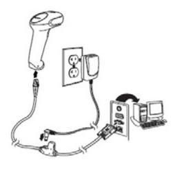
Power supplies for cabled connections
