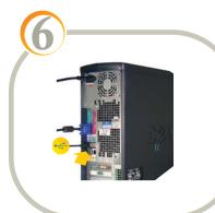
Attach the USB cable from the MSR to the USB port on the rear of the computer.
