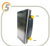
Align the MSR to the exposed mounting holes. Screw the MSR to the monitor using a Phillips screwdriver.
