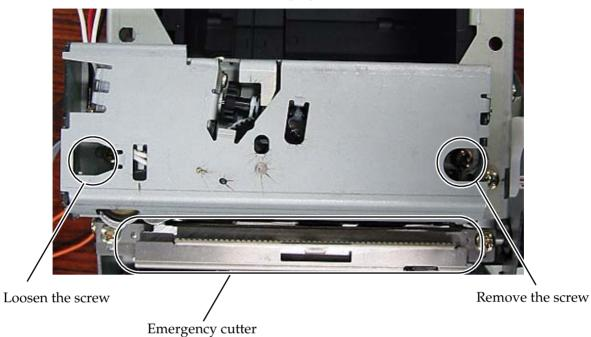
5. Lift the top of the cutter unit upward towards you and remove from the dowel.
