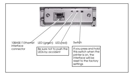
Before connecting any of the cables, make sure that both the printer and the host computer are turned off.
