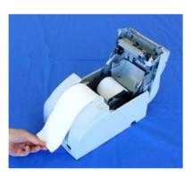
7. When using 2-ply roll paper, pull out the roll paper to the bottom front of the printer as a guide, as shown in left.
