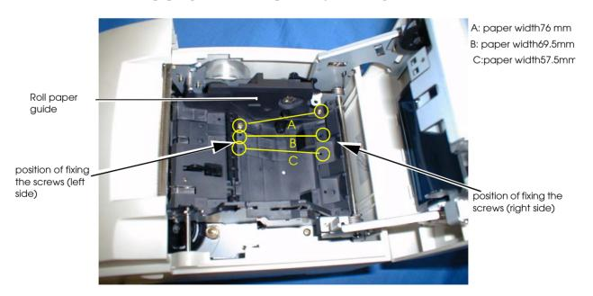
4. Push the roll paper guide on the appropriate width (See figure above.)
