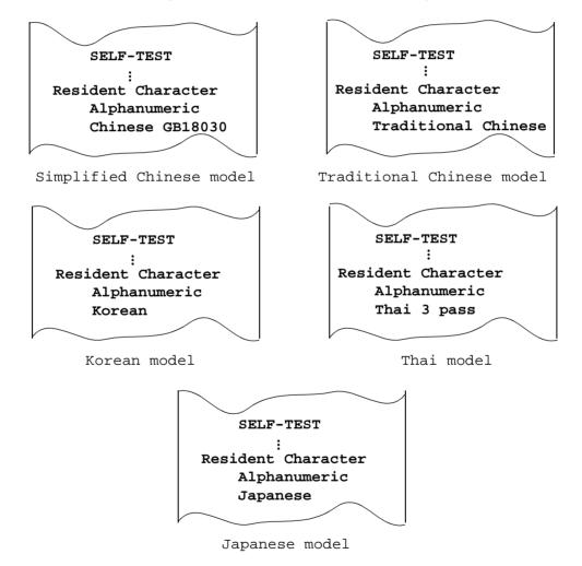
Result of SELF-TEST and printer model
