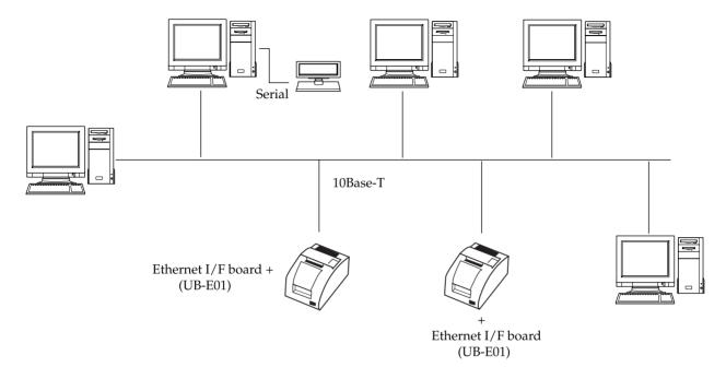
TM printers are connected to a network via a hub using an Ethernet cable.
