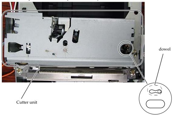
6. When you select partial cut (default), you have to adjust the dowel to the right, as shown. When you select full cut, you have to adjust the dowel to left as shown.
