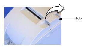
1. Turn on the printer and open the roll paper cover by using the tab, as shown.
