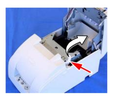
3. Type A only: Remove the take-up spool, and open the unit by using the unit open lever, as shown; then remove the used roll paper core.
