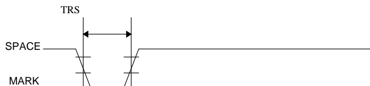
Figure 2.1.1 Minimum Reset Pulse Width (pin 6)
