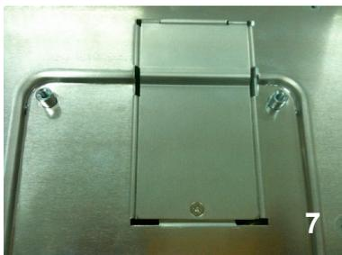
1. Unscrew 2 M3 screws (64DA30104-100B) and remove MSR.
