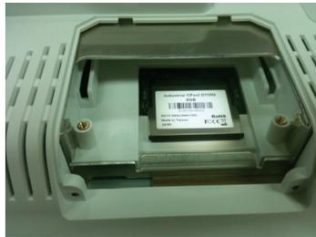
1. Unscrew 2 M3 screws (64D030060-200T) and remove the HDD cover.
