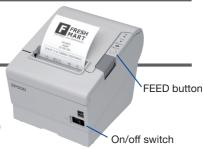
(...) Select Modus by pressing Feed button. Continue SELF-TEST: Less than 1 second Mode Selection: 1 second or more
