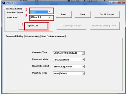
Please then follow the steps as shown in the above figure, the baud rate will show on states page of VFD module (Note: You may check it when power on VFD module), then click "Open COM" button.
