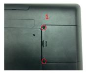
2. Remove the 2 screws from the hard drive bracket
