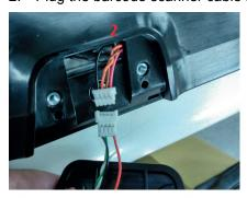
3. Install the barcode scanner with 2 screws
