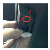
3. Plug the MSR cable into the MSR connector
