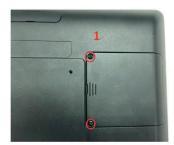
2. Remove the 2 hard drive bracket screws then remove the hard drive bracket
