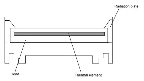
Figure E.1 Print Head Thermal Elements
