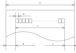
$a = 57.5 \pm 0.5 \text{ mm} (2.26 \pm 0.02")$   $b = 0.141 \pm 0.05 \text{ mm} (.056 \pm .002")$   $c = 50.8 \pm 0.2 \text{ mm} (2.00 \pm .008")$   $d = 3.7 \pm 0.2 \text{ mm} (0.15 \pm 0.079").$   $e = 3.0 \pm 0.2 \text{ mm} (0.12 \pm 0.079").$ [All the numeric values are typical.]
