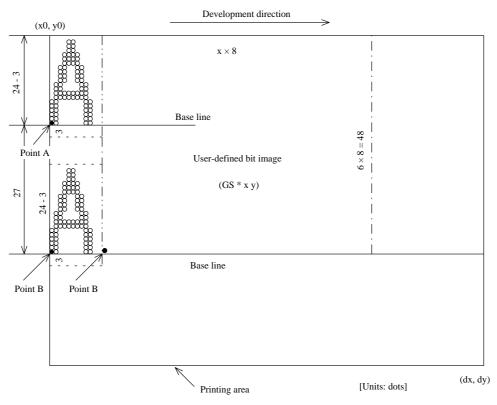
Figure 3.12.4 Downloaded Bit Image Developing Position
