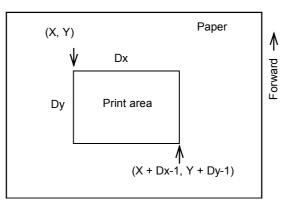
• This printable area for this printer is approximately for 80 mm paper width model; 72.2 mm {512/180"}, for 58 mm paper width model; 50.8 mm {360/180"} in the horizontal direction and approximately 117.3 mm {1662/360"} in the vertical direction.
