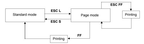
Figure 3.12.1 Shifting Between Standard Mode and Page Mode
