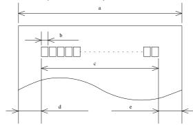
a =  $79.5 \pm 0.5 \text{ mm} \{3.13 \pm 0.02"\}$ b =  $0.141 \pm 0.05 \text{ mm} \{0.056 \pm .002"\}$ c =  $72.2 \pm 0.2 \text{ mm} \{2.84 \pm .008"\}$ d =  $3.7 \pm 0.2 \text{ mm} \{0.15 \pm 0.079"\}$ e =  $3.7 \pm 0.2 \text{ mm} \{0.15 \pm 0.079"\}$ [All the numeric values are typical.]
